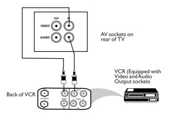
You can view the playback of VCR tapes (Video Disc players, camcorders, etc.) by using the AUDIO and VIDEO INPUT sockets on the rear of the TV.
